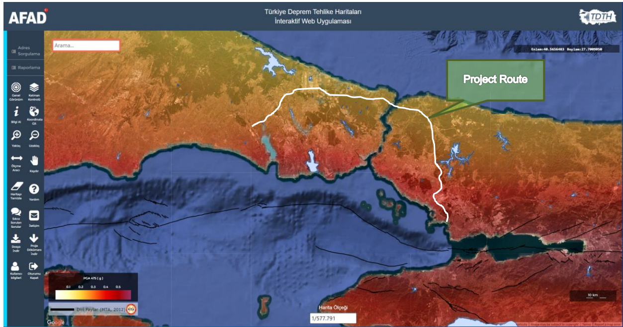
Figure 4-7 Project Route Peak Ground Acceleration (PGA 475)
